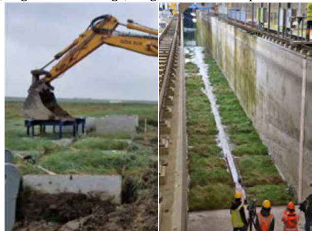
Figure 1: Obtaining marsh blocks from the field (left) and Delta Flume filled with marsh blocks (right).
